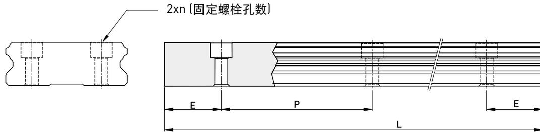
$$L = (n - 1) \times P + 2 \times E \quad \dots \dots \dots \text{Eq.2.3}$$
