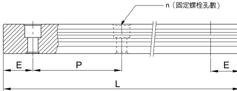
$$L = (n - 1) \times P + 2 \times E \quad \dots \dots \dots \text{Eq.2.1}$$
